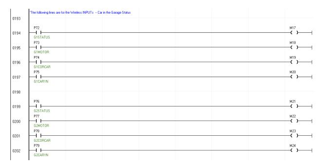
Figure 5.6 PLC Logic for Car in the Garage Status
