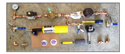
Figure 3.6 Items Needed for the Water Meter and Electric Shut-Off Valve Installation
