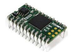
Figure 4.9 CB320 Microprocessor and PLC on a Chip
